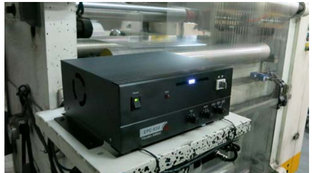
Controller Series 83 is installed on Printing Machine by Desktop
